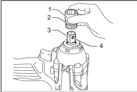
► 1. Impact socket 2. Hole 3. Square drive 4. Detent pin
