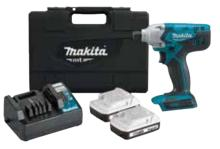
Max. capacities standard bolt M5 - M14 Max. capacities M5 - M12 high tensile bolt 0 - 2,400rpm No load speed Impact rate 0 - 3,000rpm Max. tightening torque 135Nm 6.35mm (1/4") Hex Drive shank Overall length 173mm Skin weight 1.1kg 1.5kg Weight (with battery) 18V G-Series Voltage
