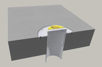
Reduce your waterproofing problems by simply rebating the outer flange into the subfloor prior to waterproofing.
