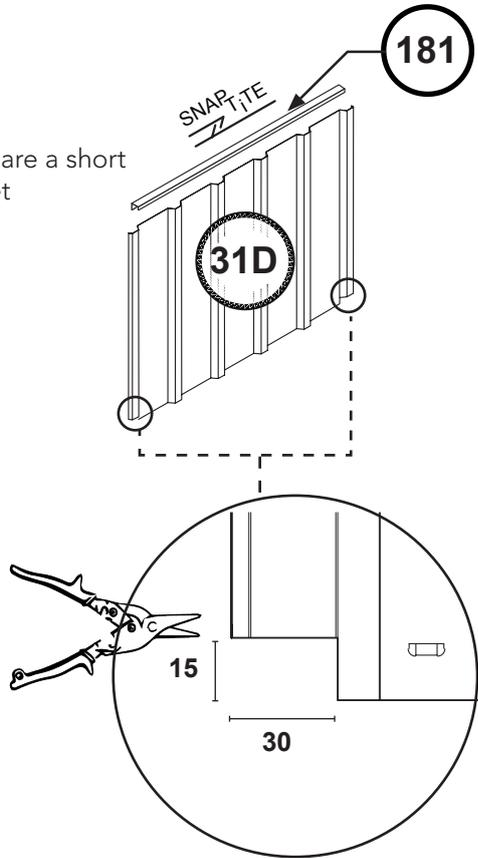
Notch out both bottom corners as shown using tinsnips.
