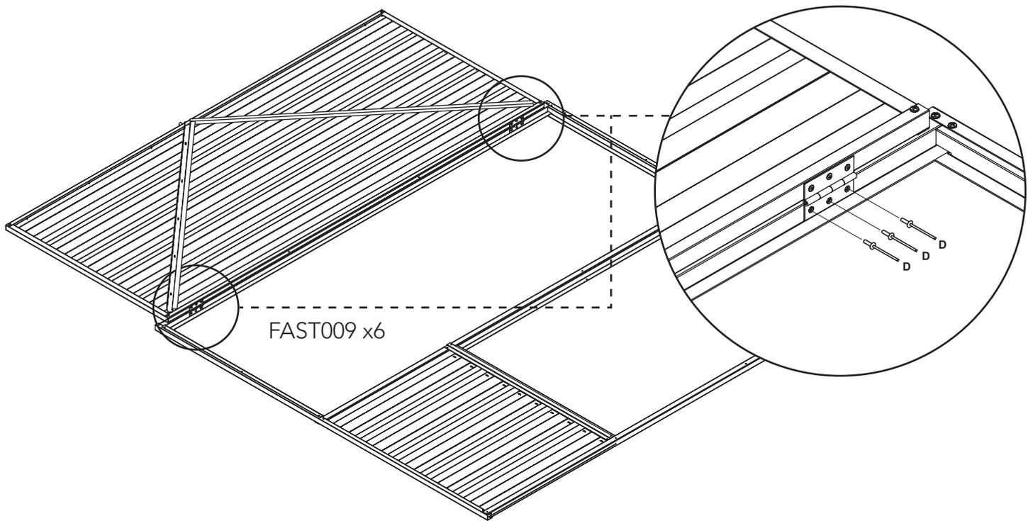
Lay the LEFT SIDE PANEL face up and lay the DOOR PANEL down in the open position on top as shown.
