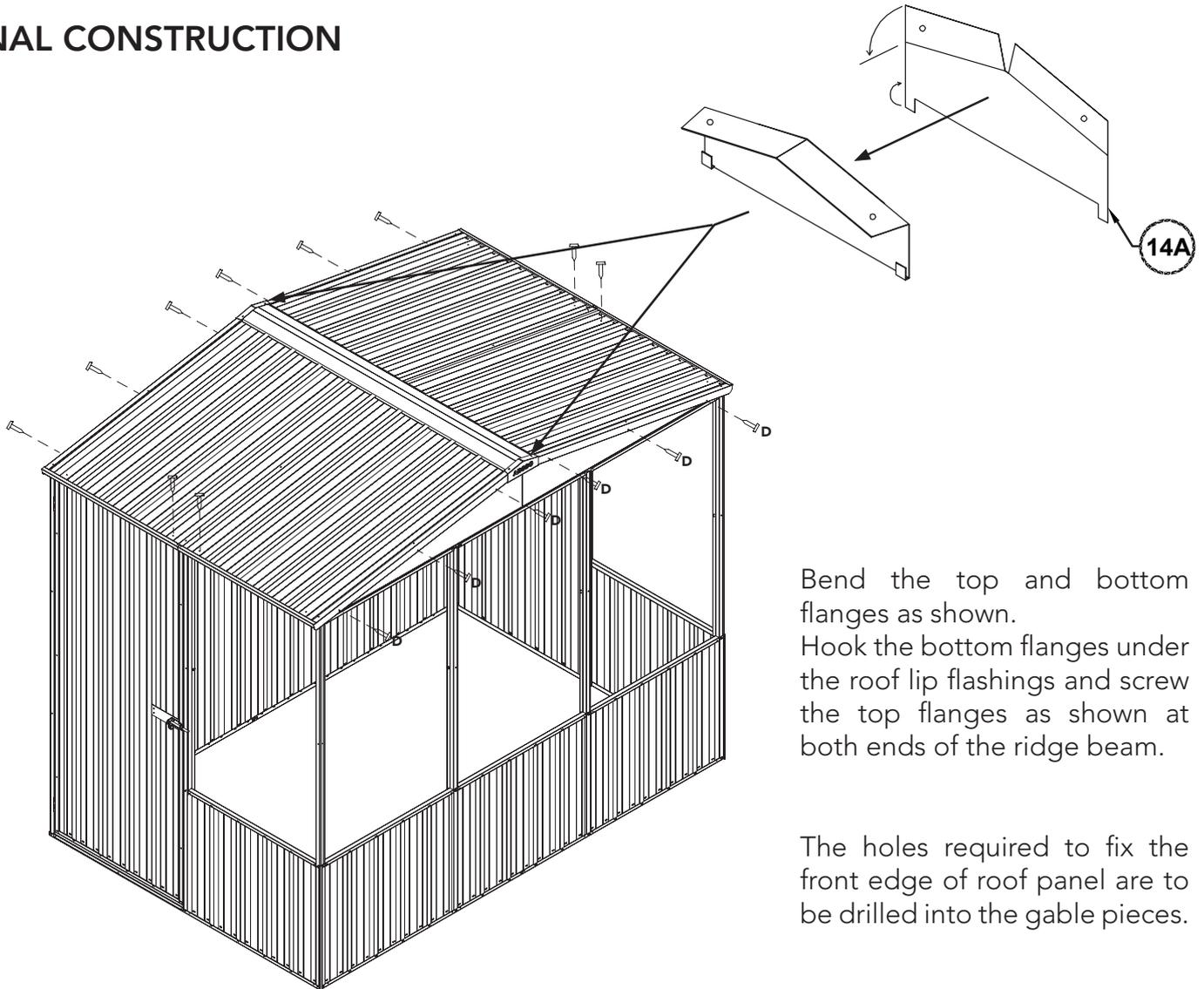
Bend the top and bottom flanges as shown. Hook the bottom flanges under the roof lip flashings and screw the top flanges as shown at both ends of the ridge beam.
