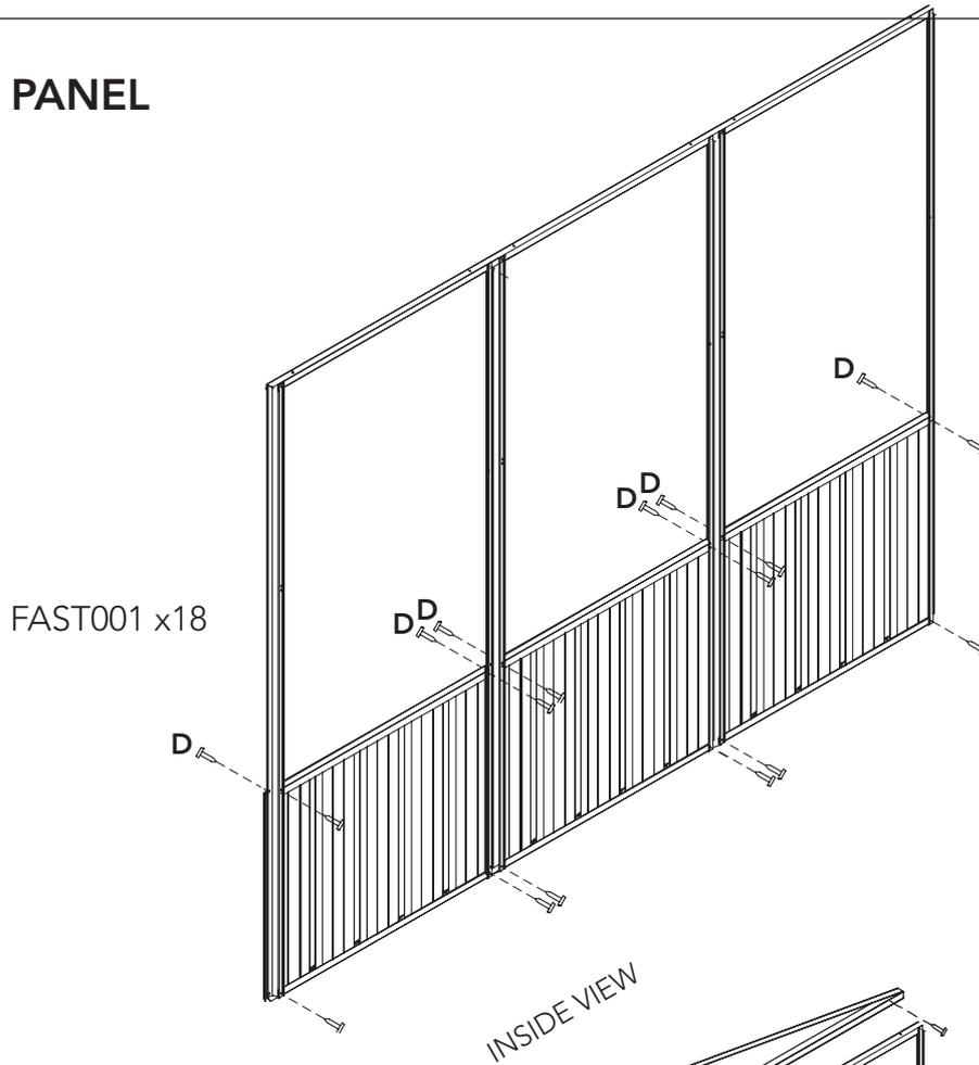
Fix the jambs from the inside of the front panel as shown.
