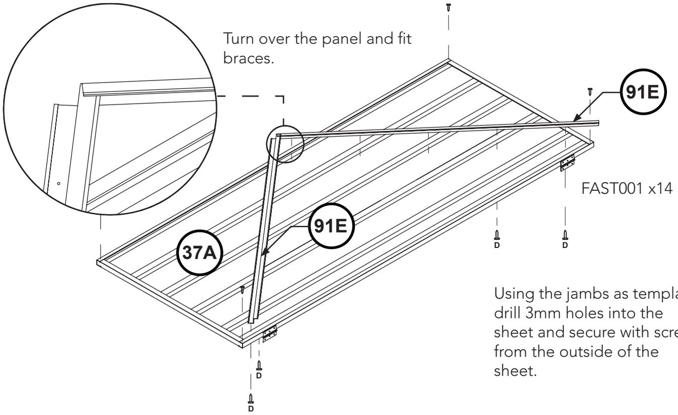
Using the jambs as templates drill 3mm holes into the sheet and secure with screws from the outside of the sheet.
