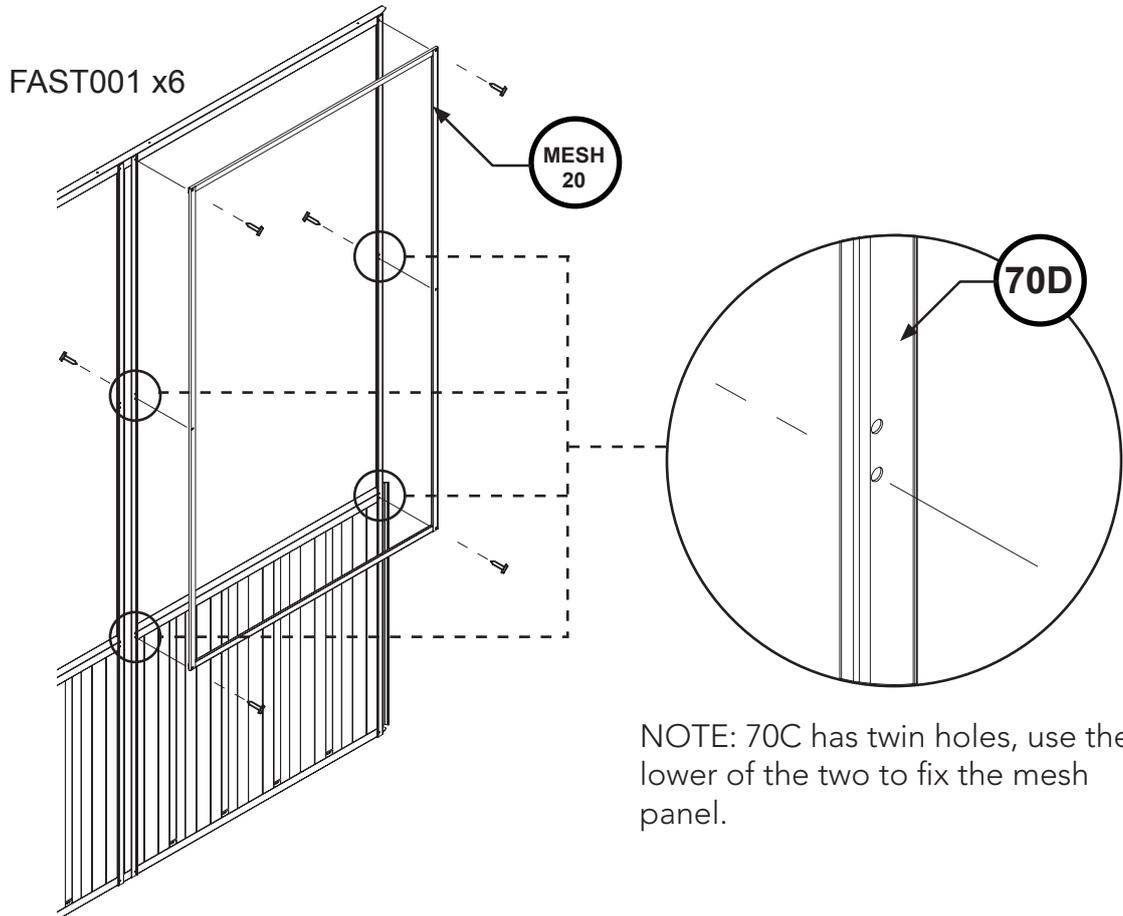
NOTE: 70C has twin holes, use the lower of the two to fix the mesh panel.
