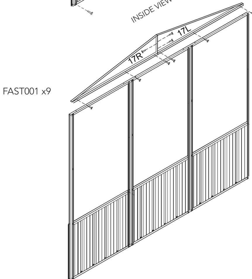
Join the gable panels 17L and 17R and move into position as shown.
