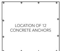
Each anchor consists of one nut, bolt, M10 dynabolt and steel angle.
