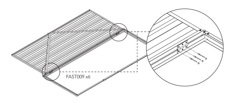
Lay the LEFT SIDE PANEL face up and lay the DOOR PANEL down in the open position on top as shown.
