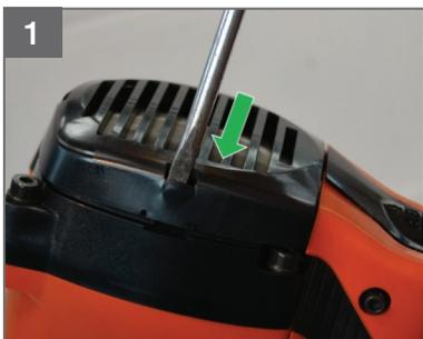
1 Using a flat bladed screw driver, remove grill #1 and filter #2
