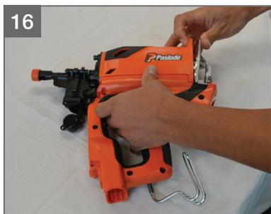
16 Carefully align head and fan blade. Caution: avoid bending fan blades during reassembly
