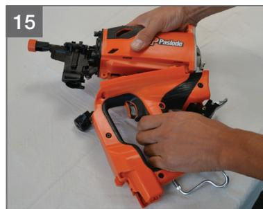
15 Carefully replace handle assembly. During reassembly, ensure wiring does not get pinched.
