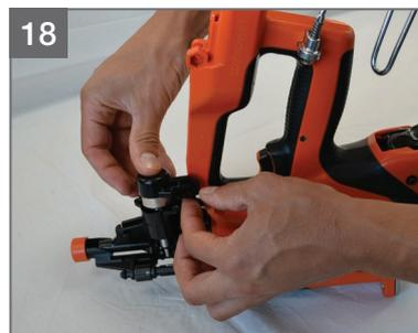
18 Replace spring #54, bumper #56, magnet #55, housing cover #57 and screws #58
