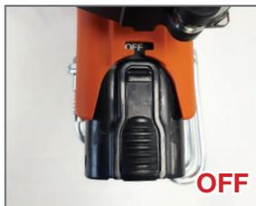
ON/OFF SWITCH. Battery has 2 secure lock positions: engaged and disengaged
