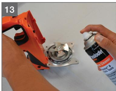
13 Spray and allow to stand for 30 seconds, then spray off the deposits, use cloth as needed
