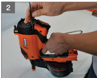
2 Take off head cap, undo cap screws #3
