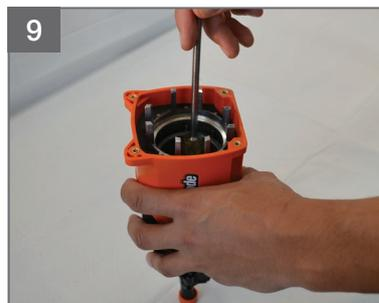
9 Push drive blade piston assembly to the bottom of the cylinder #24
