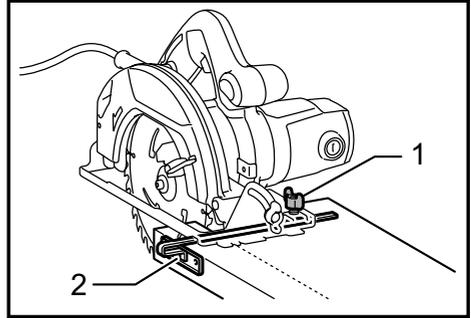
► 1. Clamping screw 2. Rip fence (Guide rule)
