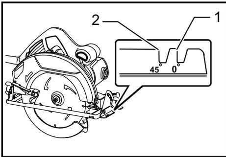
► 1. Cutting line (0° position) 2. Cutting line (45° position)
