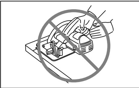
9. **Never force the saw. Push the saw forward at a speed so that the blade cuts without slowing.** Forcing the saw can cause uneven cuts, loss of accuracy, and possible kickback.
