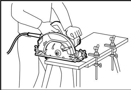
Hold the tool firmly. The tool is provided with both a front grip and rear handle. Use both to best grasp the tool. If both hands are holding saw, they cannot be cut by the blade. Set the base on the workpiece to be cut without the blade making any contact. Then turn the tool on and wait until the blade attains full speed. Now simply move the tool forward over the workpiece surface, keeping it flat and advancing smoothly until the sawing is completed.
