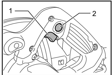
► 1. Switch trigger 2. Lock-off button/ Lock button
