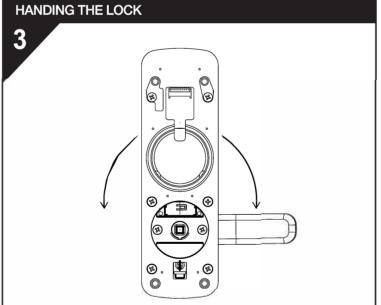
To hand the lock, on the inside of the handle, hold down on the metal slide tab -10 located towards to bottom and rotate the handle left or right depending on your selected handing -@. Ensure you hold down the tab at all times during the rotation. Rotation should be smooth, if you experience firm resistance, release the handle and slide tab and repeat handing process. Ensure you complete this for both handles.
