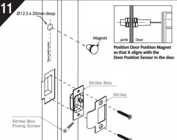
Align the DPS location onto the door jam using a pencil. Drill a 12.5mm dia x 20mm deep hole using the 12.5mm drill bit. Fit the DPS magnet into the door jam. Partially close the door and mark the position of the latch bolt to determine the striker height. Mark and mortice the door jamb to suit the strike box and strike plate. Fix the strike box to the jam and then secure the strike plate over with the timber fixing screws.
