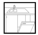
For ease of plumbing, place a dishwasher near the sink and allow a minimum 600mm space to 'house' it.
